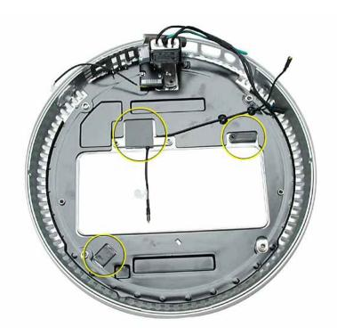
**Warning:** Whenever the logic board is separated from the bottom housing, you must install new thermal pads to three surfaces on the bottom housing. Failure to apply these pads whenever the logic board is separated from the bottom housing could cause these parts to overheat and could damage internal components.
