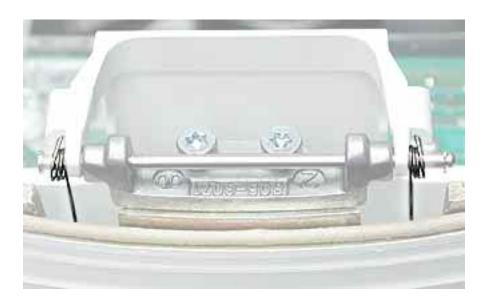
4. Remove the door hinge screws.
