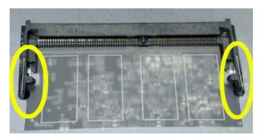
3. Gently insert the memory module into the slot. You will hear a click when the memory is completely inserted into the slot. **Note:** Make certain to push the memory module in the direction of the arrows.
