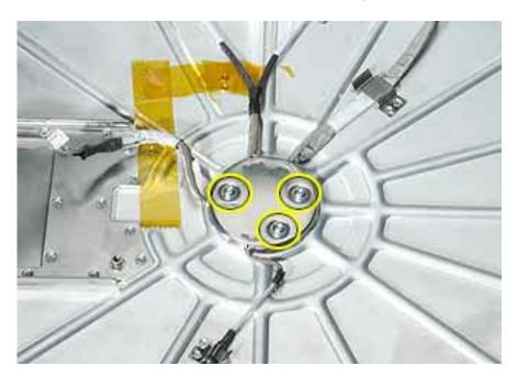
3. Loosen the four screws (shown below) that hold the panel shield to the neck assembly, and tilt the screen the opposite direction of the tilt.
