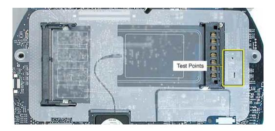
These test points provide an easy troubleshooting tool for common problems. To use each test point, put the positive probe of your voltmeter on the test point, and the negative probe on the ground pad.
