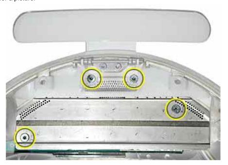
2. Slide the optical door guide off the chassis.
