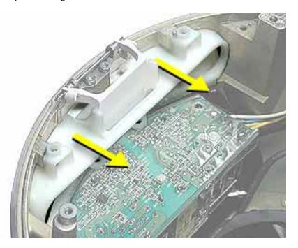
3. Carefully remove the two door springs with a needlenose pliers.
