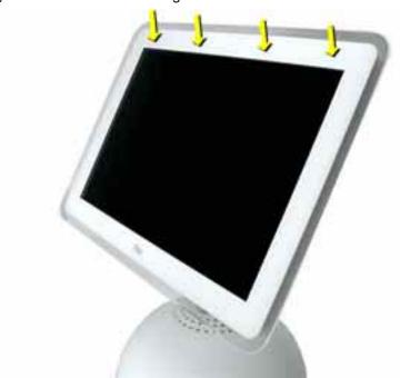
2. Holding the display, turn it over and lay the display face down on a soft cloth. Push the rear housing in the direction of the arrow. This will mate the housing and display tabs.
