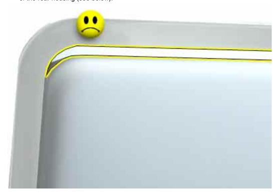
4. A properly installed display will have no white line showing across the back of the rear housing (see below), and the three display-to-housing screw holes align perfectly.
