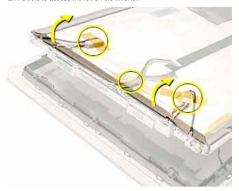
2. Peel the foil off the inverter (A). Pull the inverter off the edge of the display panel (B).
