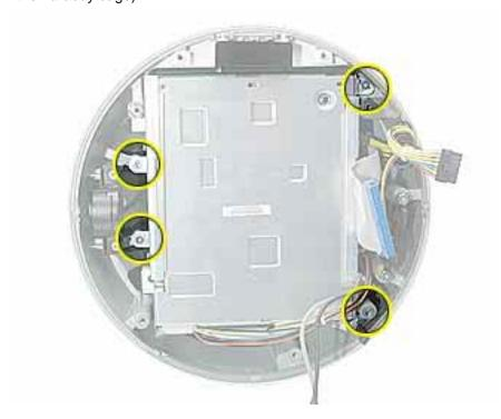
4. Remove the Airport antenna and the video cable from the plastic clip on the side of the hard drive.
