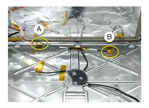
7. Remove four screws that connect the LCD display panel to the display bezel. Peel back the tape on the EMI shield to remove the LED (A) and microphone (B) cables from the display.
