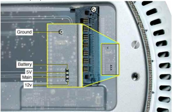
3. With the computer powered off, measure the battery voltage. Does the battery measure at least +3.5v? If no, replace the battery and reset the PMU. If the battery measures +3.5v or higher, reinstall the battery and reset the PMU as above.
