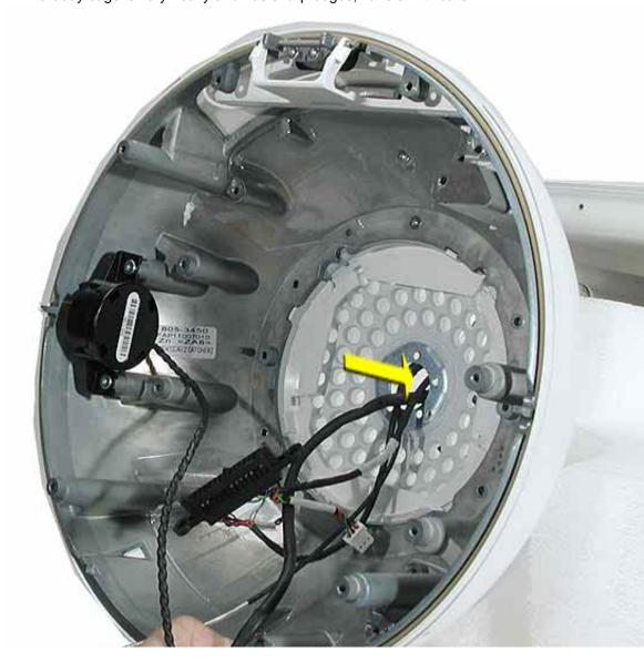
3. Pull the outer shell (with Faraday attached) away from the neck. **Note:** There is no need to remove the outer shell from the Faraday unless you are replacing the antenna or the outer shell. If you are removing the shell from the Faraday cage, go on to the next step.
