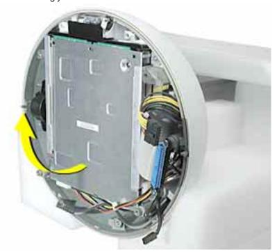
6. Peel the white wrapper up to access the screws connecting the hard drive to the carrier. Remove four screws and the hard drive.
