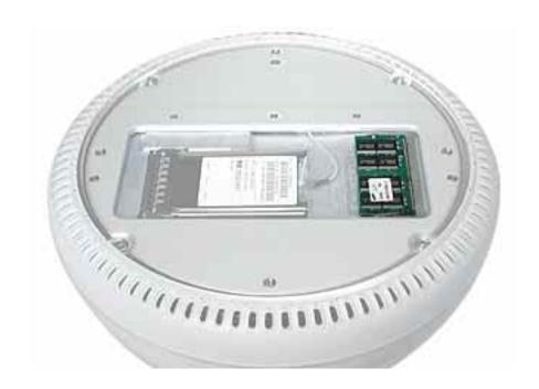
The iMac has two RAM expansion slots. The factory-installed RAM slot accepts a standard PC133 168-pin DIMM (up to 512 MB in capacity) and is accessible only by an Apple Authorized Service Provider. The user-accessible slot (shown above) accepts a standard PC133 144-pin SO-DIMM and is normally used for added RAM. Only the SO-DIMM slot is accessible by the user. A SO-DIMM for the iMac computer can contain either 64, 128, 256, or 512 MB of memory.
