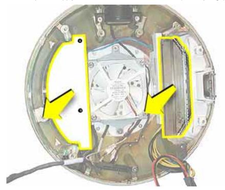
4. **Replacement Note:** When replacing the metal shield (see picture above) that sits on top of the power supply, make certain that the two shorter screws are inserted into the screw holes near the optical door. If the longer screws are inserted by mistake, the screws will scratch the top housing (circled below).
