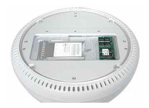
**Note:** The user-installable memory slot is identified as Slot J12 by Apple Hardware Test and Apple System Profiler.
