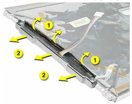
2. Remove tape and disconnect the two inverter cables (step 3 below). Pull the inverter off the edge of the display panel (step 4 below).
