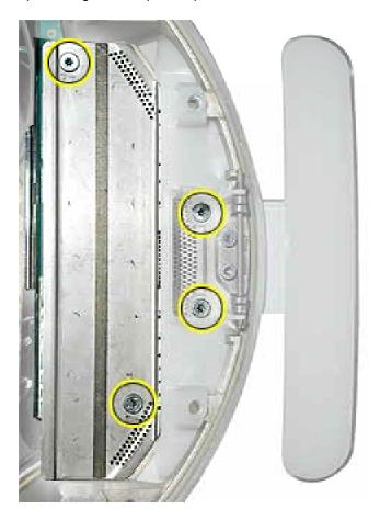
3. Remove the power supply and metal shield from the chassis (Faraday cage).
