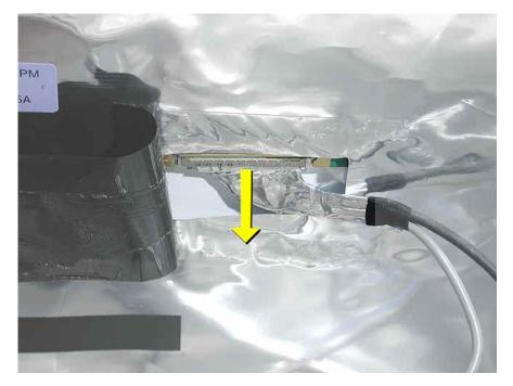
6. **Caution:** The power on LED cable (labelled A below) is fragile. Raise the top of the display to access the power on LED (A below) and microphone (B below) cables. Peel back the tape and disconnect the cables.
