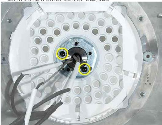
2. Carefully feed the neck cables through the hole in the Faraday cage. **Important:** The Faraday cage is very heavy and has sharp edges; handle with care.
