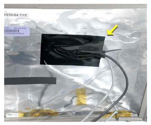
5. Disconnect the TMDS connector. **Note:** Enlarge the page to view the graphic at a larger size.
