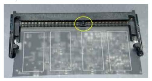
2. **Important:** Do not push the clips (circled below) when inserting memory. They are used to remove memory from the slot, not when inserting memory. These clips are fragile and can break.
