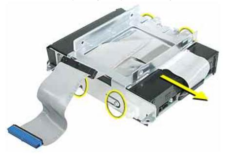
Slide the optical drive out of the carrier. Be careful of the black plastic dust filter on the carrier. It is very fragile and can rip easily if not handled properly. Note: The silver insulator is part of the carrier assembly.
