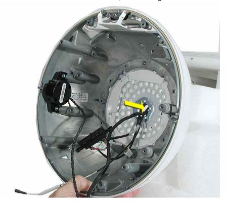
3. Next, carefully separate the outer plastic housing (with Faraday attached) from the neck.
