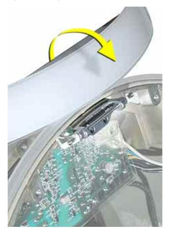
6. Slide the door and hinge off the frame. Remove the door from the base.
