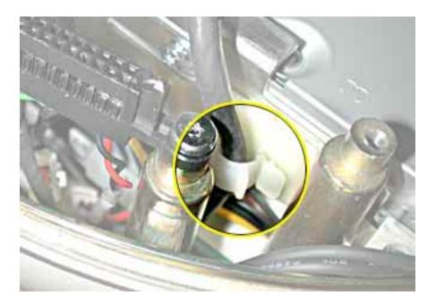
Grasp the carrier on both sides. Lift and pull the carrier in the direction of the arrow.
