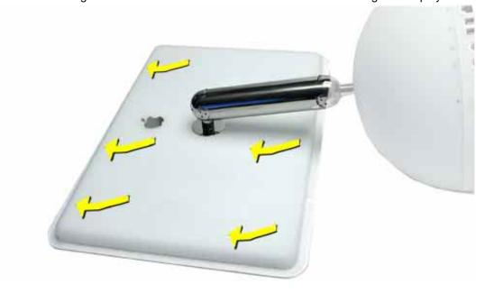
3. Check the alignment of the rear housing and the flat panel display. If the display doesn't slide into the tabs/slots on the rear housing, a white line shows around the top of the rear housing (see below).
