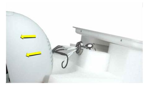
4. **Note:** Perform this step only if you are replacing the antenna or the outer shell. Remove the three screws in the base of the Faraday cage to separate the shell from the Faraday cage.
