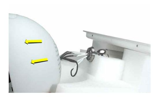
4. Remove the three screws in the base of the Faraday cage to separate the outer shell housing from the Faraday cage. **Note:** the cables would have been removed already.
