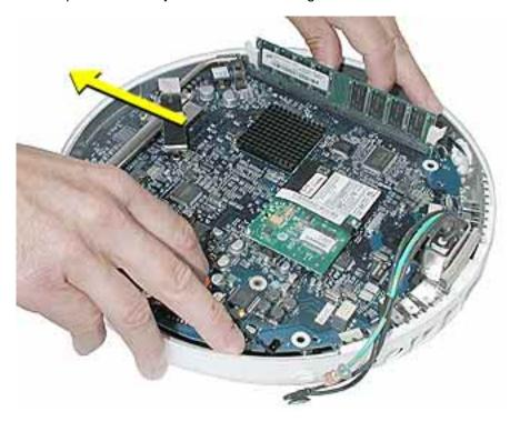
3. Remove the I/O port covers from the logic board.
