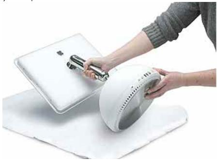
3. Loosen the four captive screws at the base of the computer and gently remove the access panel.
