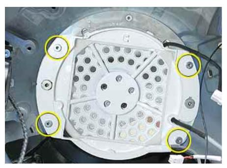
2. Lift the fan bracket from the chassis. **Note:** The fan gasket is stuck to the back side of the fan bracket.
