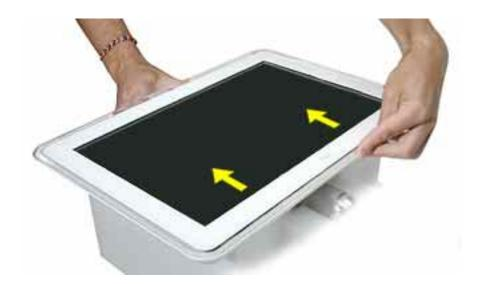
3. Caution: The power on LED cable (labelled A below) is fragile. When disconnecting display cables, be sure to raise the TOP SIDE of the display only. Carefully raise the TOP SIDE of the display and disconnect the inverter cable (B) and remove the TMDS cables (C) from the metal cable clip. Note: Enlarge the page to view the graphic at a larger size.
