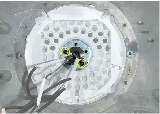
2. Carefully feed the neck cables through the hole on the vent cap shown below. Start with the blind mate connector and cables, then the long video cable
