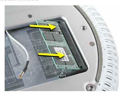
4. Press down gently on the memory until you hear it click into place under the two locking tabs (circled below) on the sides of the slot.
