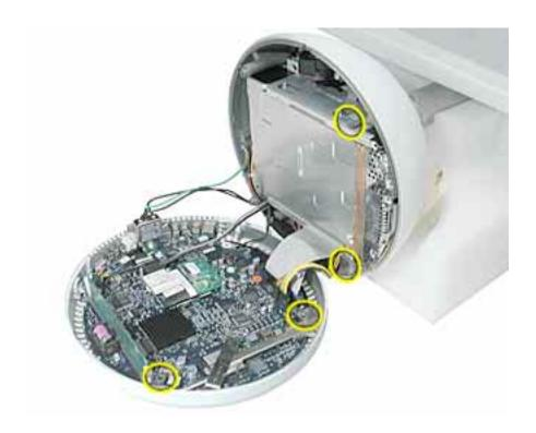
Thoroughly clean the original thermal film from the mating surfaces (circled below) of the bottom housing and thermal pipe. Use a plastic stylus to scrape the surfaces clean. Note: Do not use an abrasive material or liquid cleaner.
