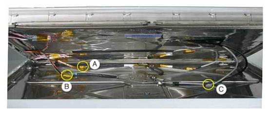
4. Raise the display to access the TMDS connector. Peel back the black tape.
