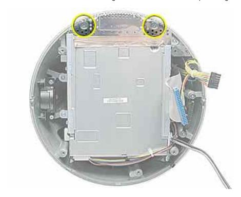
3. Remove four screws attaching the drive carrier to the metal chassis (also known as the Faraday cage).
