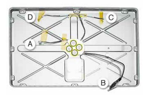
Remove tape from the neck cables and pull them through the hole in the back cover.
