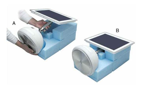
2. **Note:** The base of the computer can be rotated when servicing internal parts.
