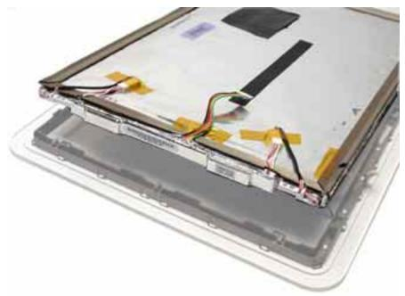
9. **Note:** Remove the inverter (refer to the next procedure) from the display if you are returning the flat panel display to Apple.
